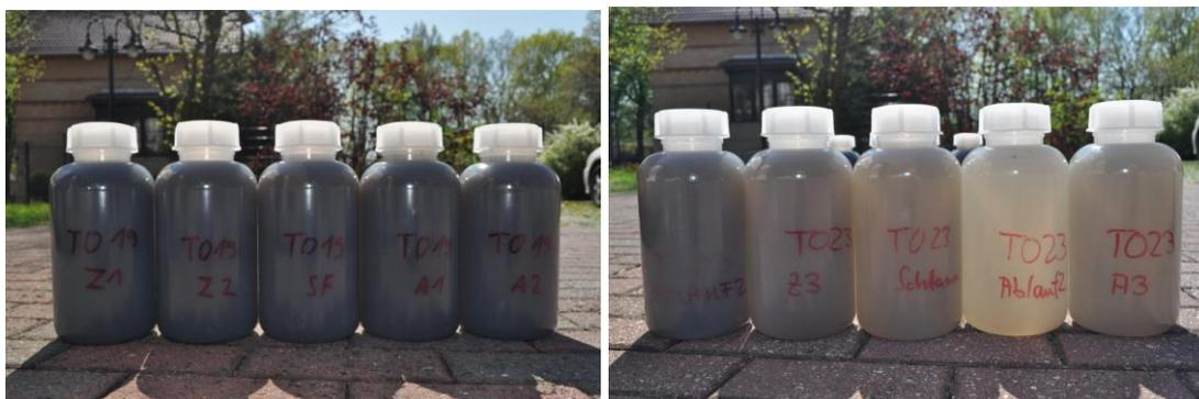
Abb. 4: Comparison of inflow/outflow, left side: inlet without INNOLET G, right side: inlet with INNOLET G
