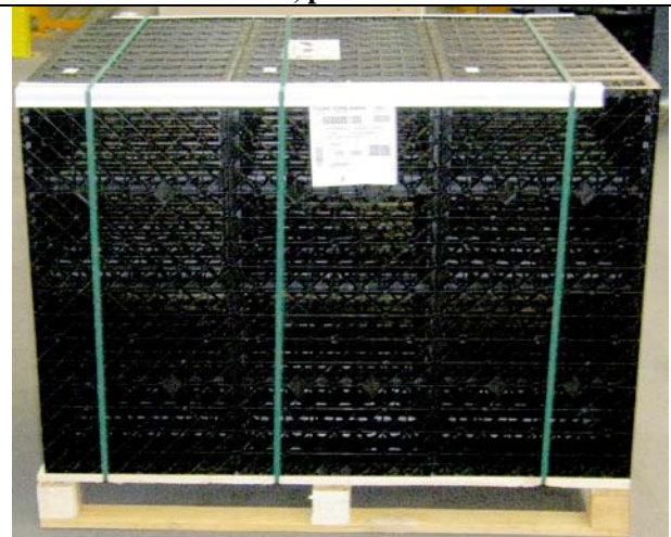
Picture 12. A product label must be stuck on the long and the short side of each pallet. The product label must contain the name, personnel number and date
