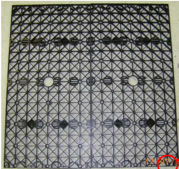
Picture 2: The single side paver prior to installation
